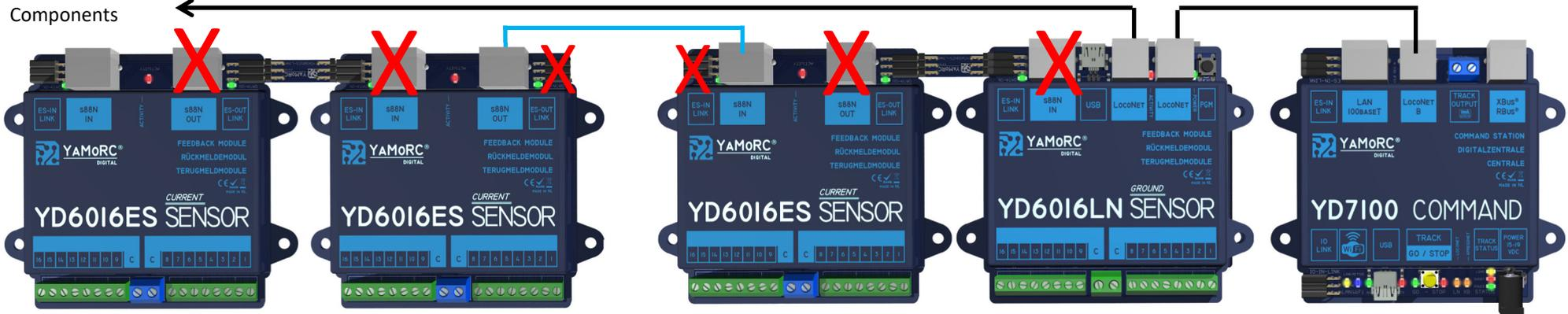
**Maximum extension:** 96 feedbacks, consisting of five feedback modules with 16 inputs each in the entire "ES-Link" line.
